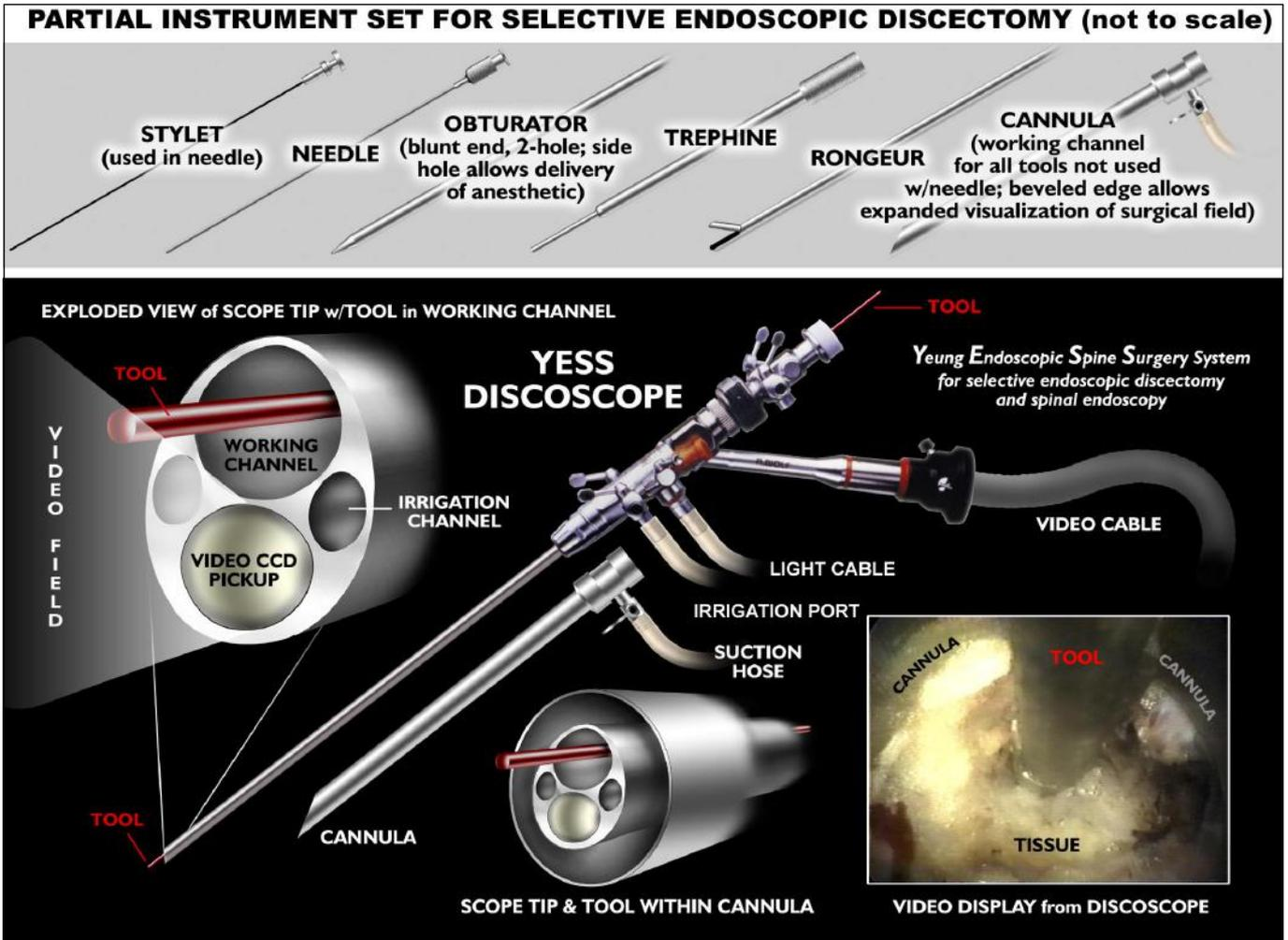
**Figure 5. The YESS™ endoscope features multi-channel irrigation and a 2.8-mm working channel. Complementary access cannulas and instruments improved visualization of the epidural space and the foramen. (Illustration by David Azarello)**
